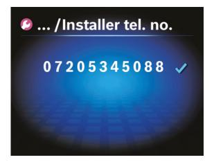
Telephone number can be added to the control display for easy contact and resolution.
